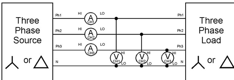
Three-phase, Four wire (3 wattmeter method)
