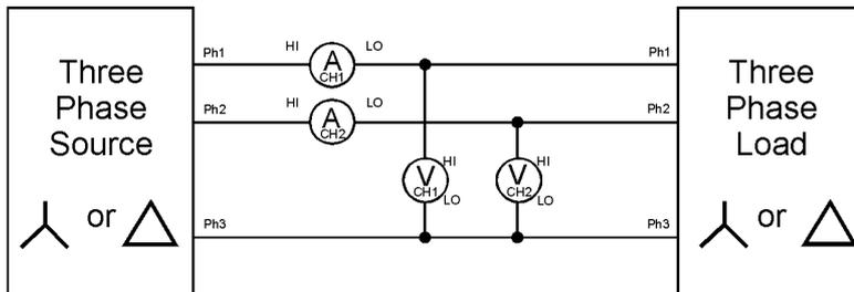
Three-phase, Three wire (2 wattmeter method)
