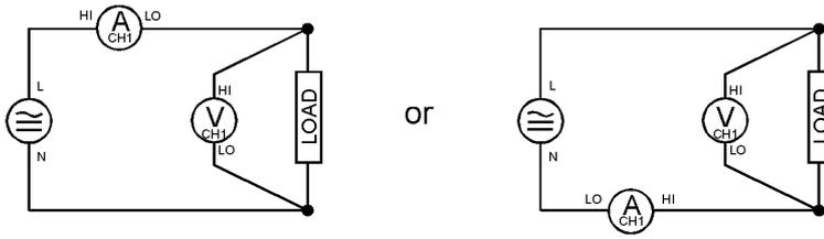
Single-phase, Two wire and DC measurements
