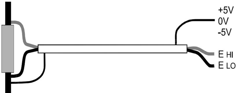
• Figure 3 External Resistive Shunt with Shielded Twisted Pair
