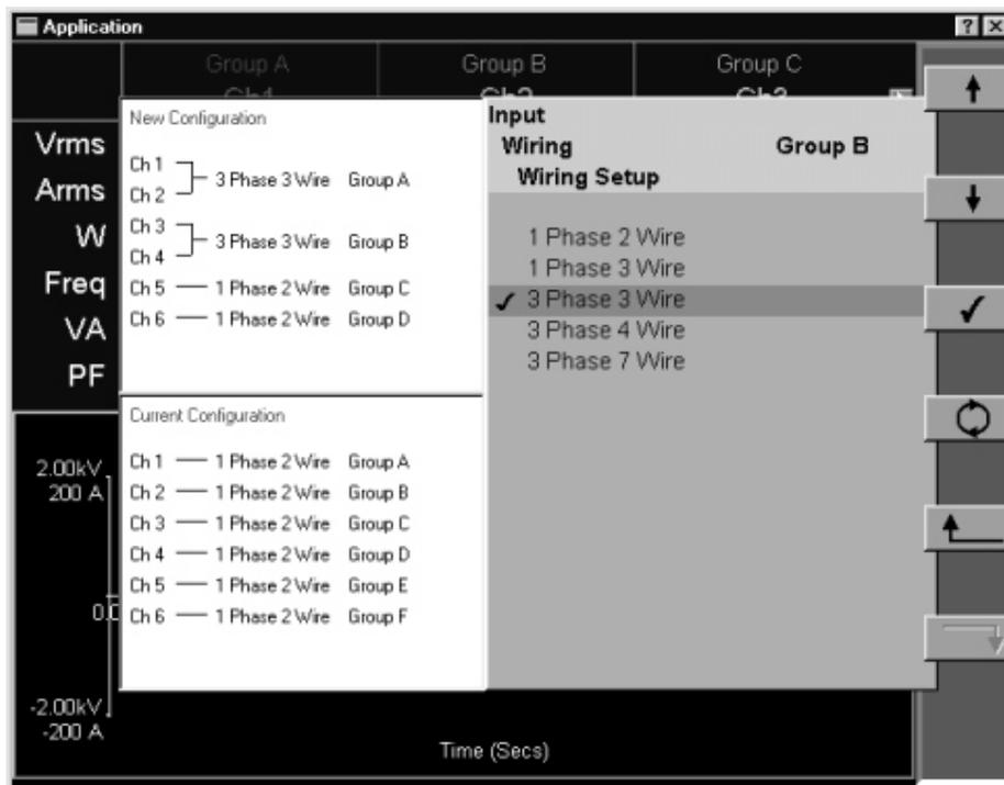
In this example, CH1 and CH2 have been grouped together to measure a 3-phase input, and CH3 and CH4 have been grouped together to simultaneously measure a 3-phase output
